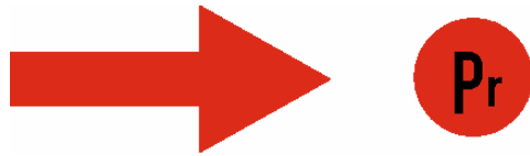
Fig.10. Information marks - flow direction and pressure output
